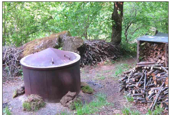
Modern metal charcoal kiln for small scale domestic use.
