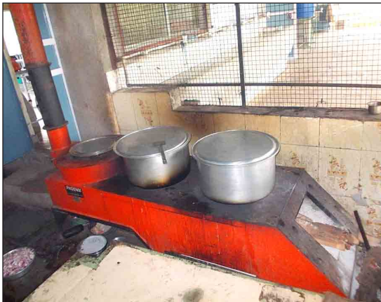
Improved design of cookstove made of cement with chimney to exterior at left. Credit: Wikimedia, Pooja Jadhav.
