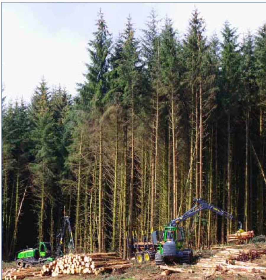
Conifer plantation being felled for timber, using the harvester at left, and the forwarder at right which carries logs to transport trucks.
