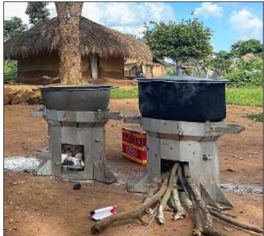
Experimental design of metal cookstove being tested in Sudan. Credit: Wikimedia, Laura Toledano.
