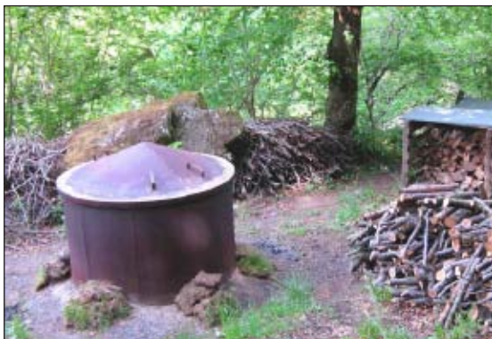
Modern metal charcoal kiln for small scale domestic use.
